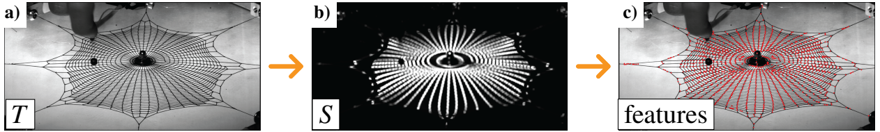
Fig. 3 Automatic feature selection in a spiderweb-like cable network. a) A template image T is established. b) T is filtered, for example, with \lambda_0 to create the score image S . c) Features are selected automatically from S with an algorithm, for example, in descending order of score, at local maxima, or with ANMS.
